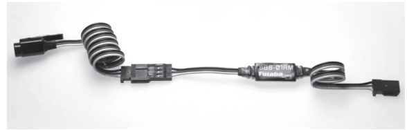
RPM-Sensor SBS01RM Magnetic No. F1732
